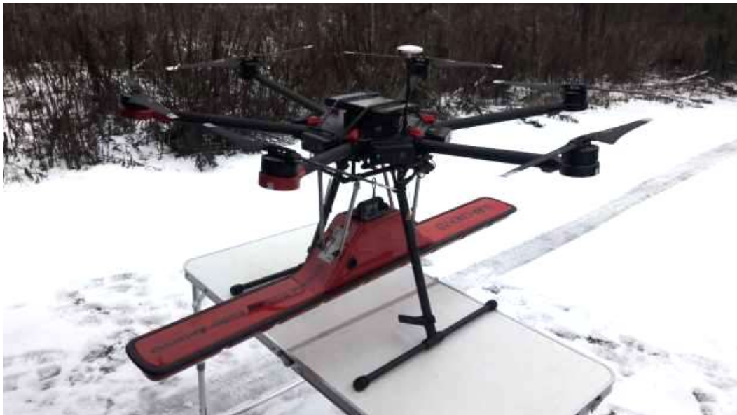
Figure 7. GPR and tablet mounted on the drone, i.e. without integration.
