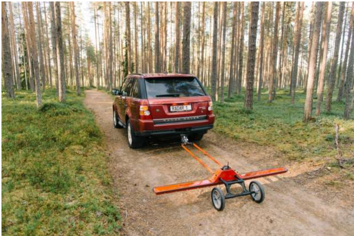
Figure 1. Cart-mounted GPR system being towed by a vehicle. © Image courtesy of Radarteam Sweden.
