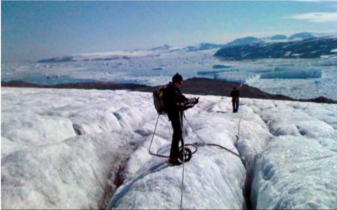
Figure 2. Before the availability of GPR mounted on a drone, searching for a missing WW2 aircraft in Greenland entailed dragging a manual dolly equipped with a GPR radar system over dangerous crevasses and perilous terrain.
