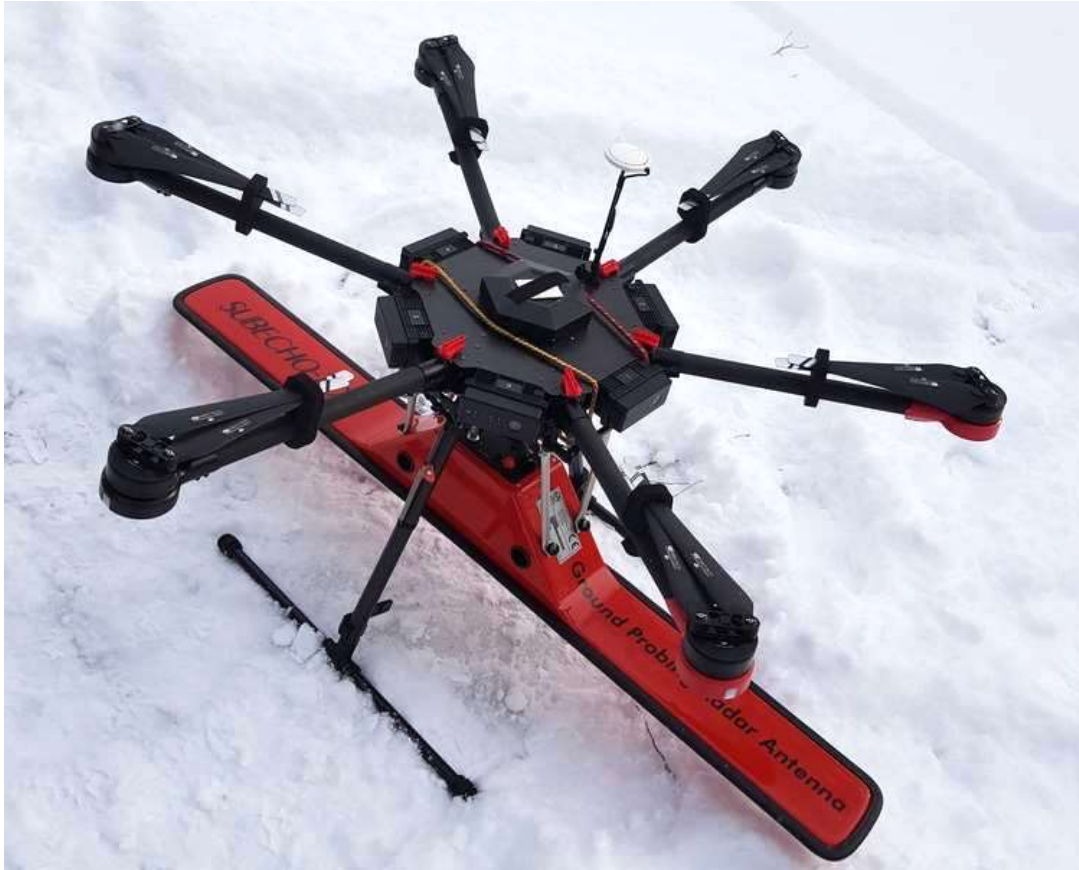
Figure 4. The GPR-drone (DJI M600Pro) integrated system.
