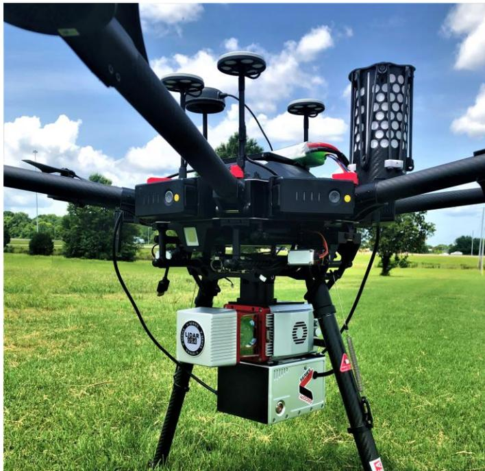
Weighing in at only 430g in a re-packable canister of only 160x75mm (HxW), the DRS-M600 is designed to auto-release using a patented, airplane-friendly, ejection mechanism within milliseconds of detecting a system failure. Effective as low as 10m with a descent of 3m/s, the equipment will land without a hard impact yet quickly enough to keep from being dragged far away.
