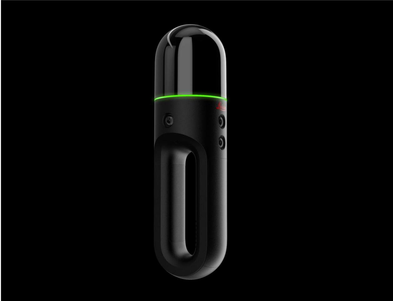
where it has been in space and will accurately follow a user's trajectory while scanning. When used with the iOS app, users can get live feedback while scanning, check the device status, or do quick data inspection.
